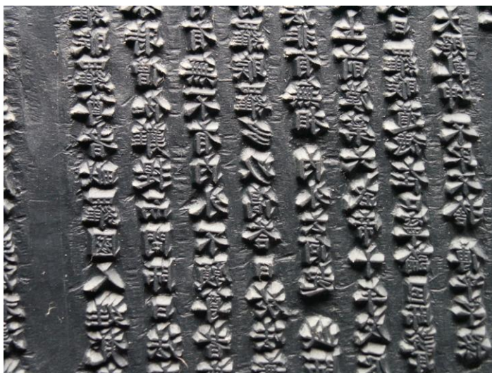
Illustration 2: Detail of a printing-block of ZTJ; scribes outlined each character on the woodblock in mirror-writing and afterwards the wood surrounding each character was chiseled out; the tool marks are still recognizable on the blocks; the wood (birch tree) is of exceptional hardness and was especially prepared for carving during a process lasting several years (photograph by C. Anderl).
